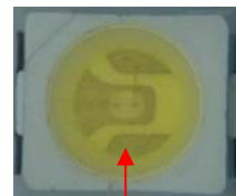
Sulfide materials, stent Bowl Cup silver layer black 硫化后支架碗杯银层变黑
